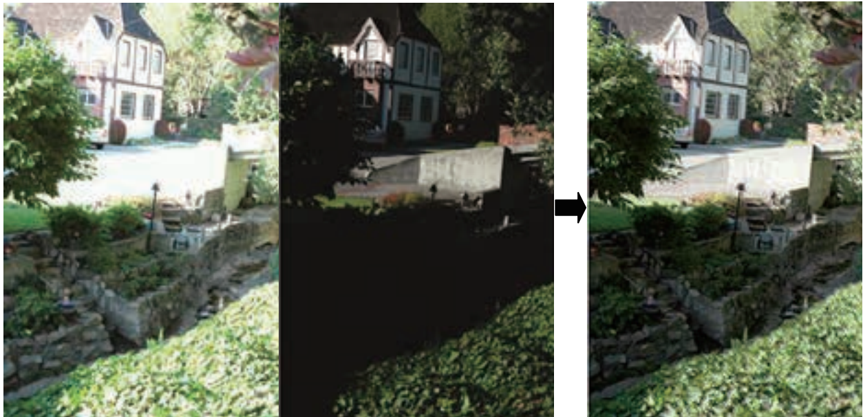
Figure 6. Simulation Effect of Hikvision WDR Technique
